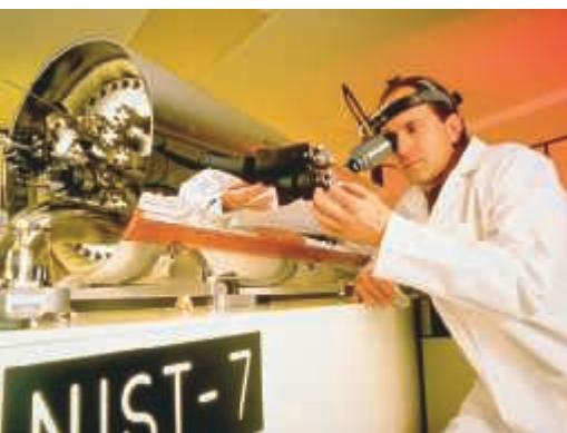
▲ FIGURE 1-3 This atomic clock, which keeps time on the basis of radiation from cesium atoms, is accurate to about two ten-millionths of a second per year. (How much time would it take for it to gain or lose an hour?)
